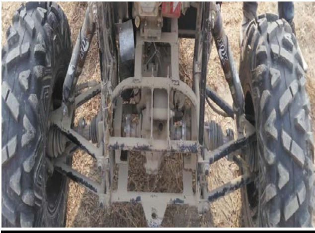
Fig.11 Over all arranged transmission line
